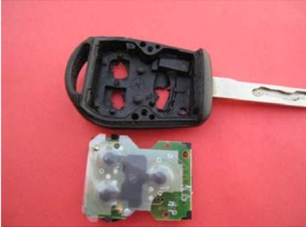
Separate electronic board with glued plastic protection cover. If clear cover is loose, re-glue it with super glue at the corners. Use very small dots of glue.
