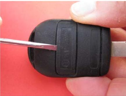
with flat screwdriver lift plastic cover positioned on the back of remote. You will uncover two screws which hold top and bottom part together
