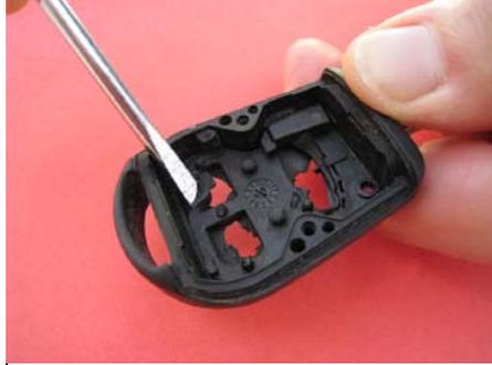
Use flat screwdriver to shave of old rubber layer. Do it gently so you do not damage hard shell.
