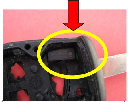
**Important:** please be careful not to damage **Coding Chip** located in the key part of the plastic cover at the bottom right corner
