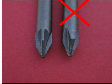
**Do Not use Phillips screwdriver** (shown on the right) as you may damage screws
