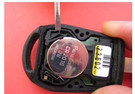
Gently lift electronic board to separate it from the top key part of the plastic cover
