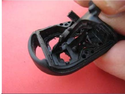
Once rubber starts parting from plastic cover, start pulling it gently and detach it. You should end up with cover looking like one in the picture above clean from old rubber remains
