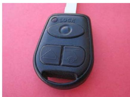
Once your new silicone pad is fitted in you need to close your remote by placing electronic parts in, covering it with bottom part of remote and screwing screws in using pozidriv driver.
