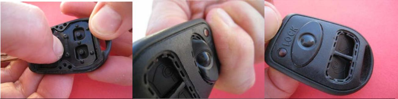
You have to push it in from inside the button using your thumb nail and manipulate it into position till whole button comes thru an opening.
