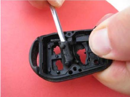
Continue rubber removing process using flat screwdriver with gentle shaving motion
