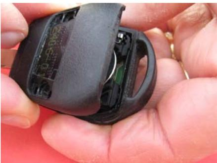
Lift back cover to uncover electronic board with immediately visible battery. After opening you will end up with parts as pictured above
