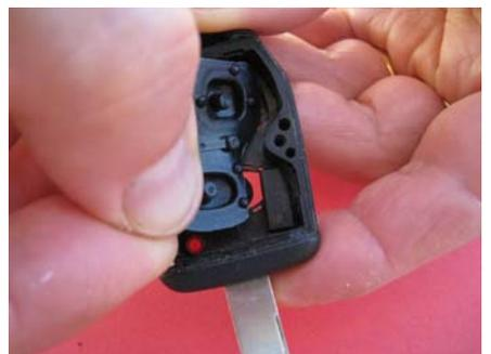
To fit new pad in you need to slide edge of oval button under the coding chip first.
